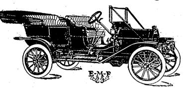
Five Passenger Touring Car, Full Equipment 4 Cylinders.30H.P.,108in. Wheel Base, 32 x 3 1-2 Tires, Magneto and Dry Cells, Sliding Gear, Selective Type, Vacuum Oiling System.
