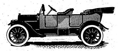
Five-passenger, four cylinders, long stroke,  $3\frac{1}{2}$  inch bore x 5 inch
